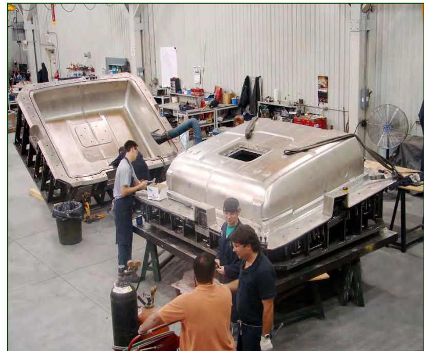
Assembly of Nickel Shell to Mold Base
